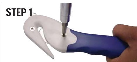
Use a screwdriver to undo both screws.
