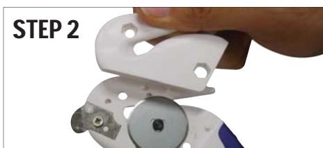
Turn cutter over and lift up cover to reveal rotary blade.
