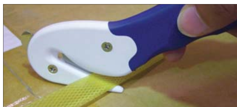
For optimum results cut strapping on a 45 degree angle.
